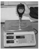
Apply a force N to the tip. When readings are almost unchanged, press the key 'MAX' to hold the reading P which should satisfy the equation below.
